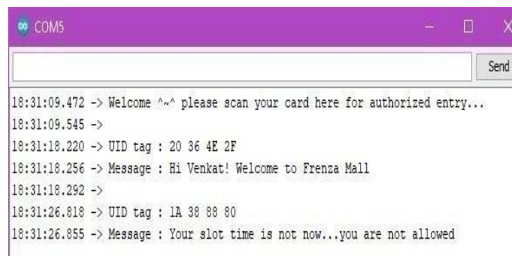
Figure 9. By scanning RFID card or tag using RFID reader, the serial monitor shows whether the customer have the authority for checkin.
